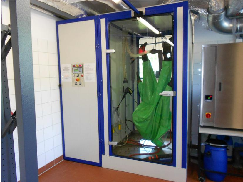
Cleaning, Disinfection and Drying Cabin for a maximum of 2 treatment spaces.
